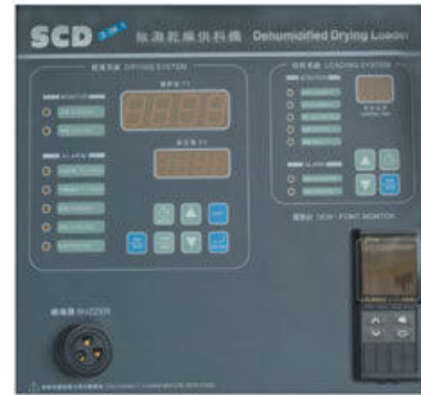
Optional panel with dew-point monitor
