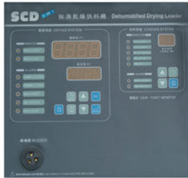
Standard panel without dew-point monitor
